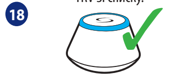
Gateway stop flashing and turn to steady blue color which means pair process has been finished.
