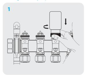
Attach the THB to the underfloor heating manifold thermostatic valves on the return bar. Ensure it is fully tightened to the manifold. Actuator is in fully open position out of the box for easy installation.
