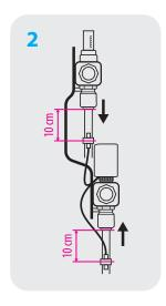
Attach the two pipe temperature sensors, one on the flow pipe and the other on the return pipe. Ensure they are placed facing forward, 10cm down from the manifold.
