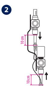
Attach the two pipe temperature sensors, one on the flow pipe and the other to the return pipe.
