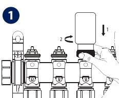
Attach the Auto Balancing Actuator to underfloor heating manifold thermostatic valves, on the return bar. When installing the THB23030/THB2430 ensure it is fully tightened onto the manifold. Actuator is in fully open position, out of the box, for easy installation.
