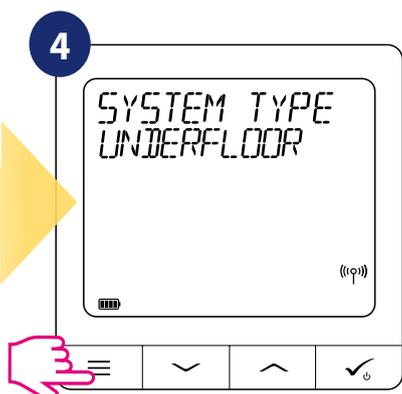
Press button for 3 seconds to expand "SYSTEM TYPE" menu.
