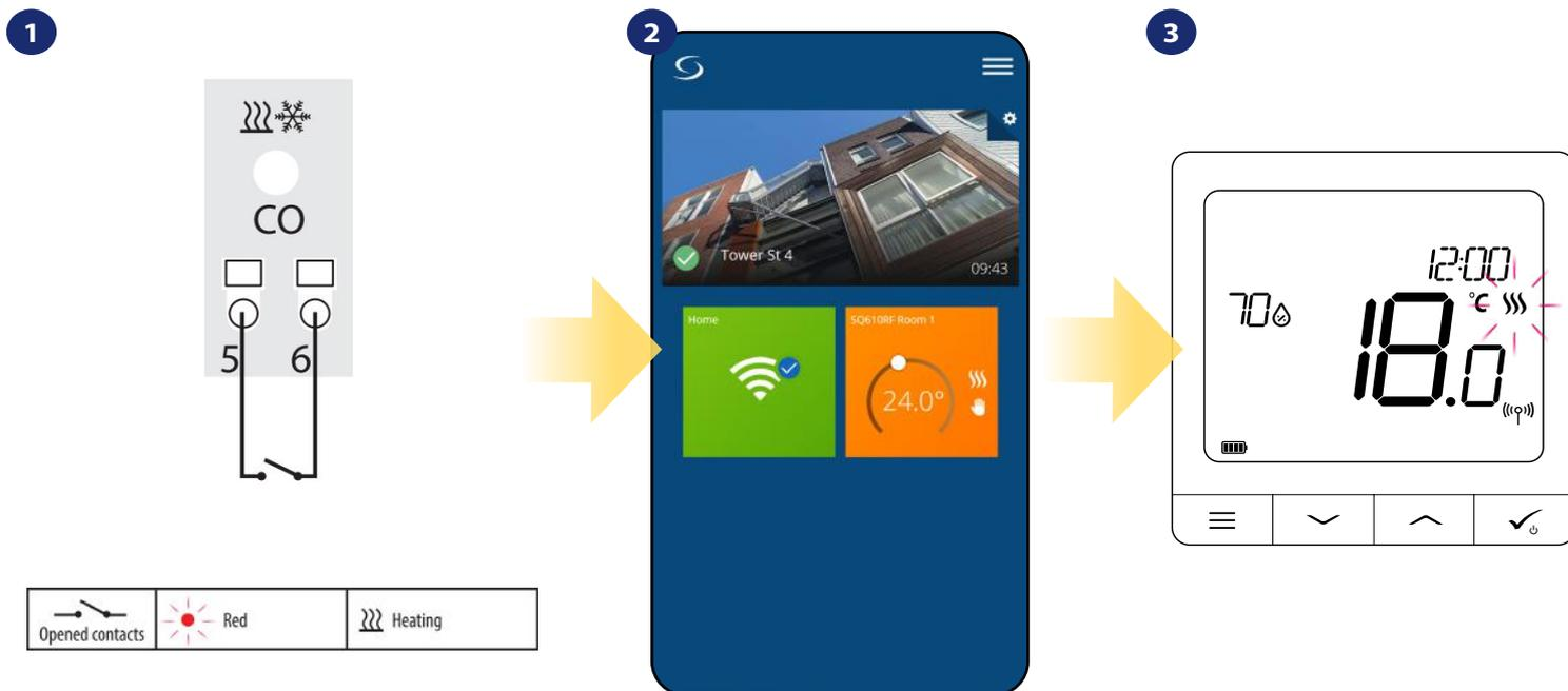
When there is no jumper at „CO” terminal KL08RF is automatically working in heating mode.
