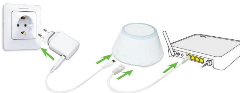
To begin the pairing process the Gateway should be plugged into the power supply and connected to the Internet. Also, make sure that the UGE600 is added to your Salus Smart Home App. For the installation of the Universal Gateway, please refer to the UGE600 manual on [salus-manuals.com](http://salus-manuals.com)
