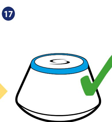
Gateway stop flashing and it turn to steady blue color which means pair process has been finished.
