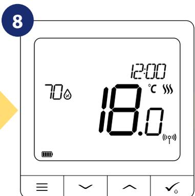
When thermostat is successfully paired main screen will be displayed.
