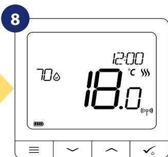
8 When thermostat is successfully paired main screen will be displayed.
