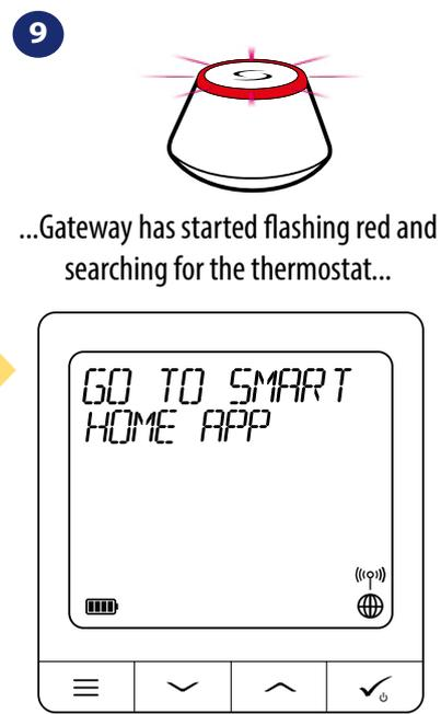
9 ...Gateway has started flashing red and searching for the thermostat...
