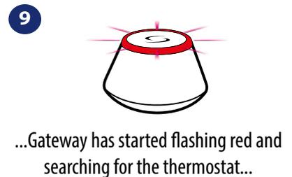
9 ...Gateway has started flashing red and searching for the thermostat...
