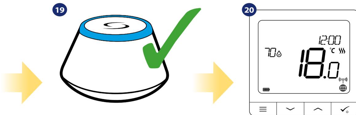
Gateway stop flashing and turn to steady blue color which means pair process has been finished.
