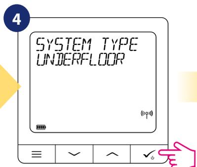
4 Select system type: UNDERFLOOR, press
