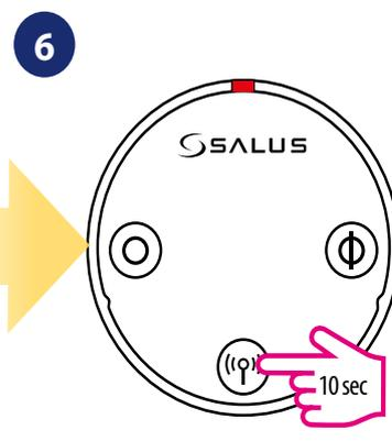
You can pair up to 6 TRV's with 1 thermostat. All TRV's have to be within the same room with thermostat.
