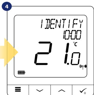
In the **Identification mode** thermostat's display will start flashing „IDENTIFY” information for 10 minutes.
