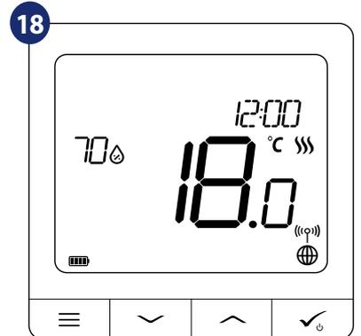
After that thermostat will display main screen. Congratulations! You successfully configured SQ610RF Quantum Thermostat with RX10RF boiler receiver.
