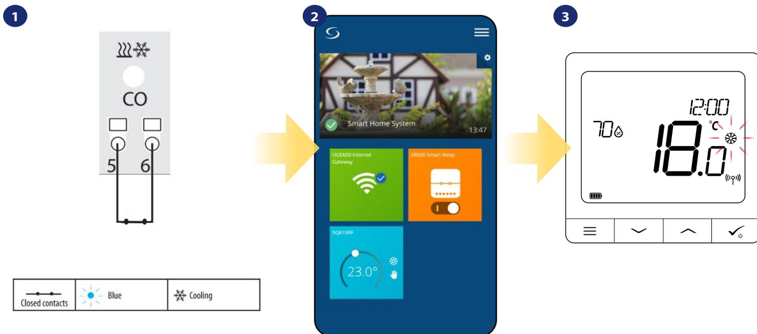
When there is jumper at „CO” terminal KL08RF is automatically working in cooling mode.
