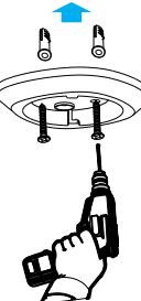
Install the bracket using the screws or the provided double-sided tape.
