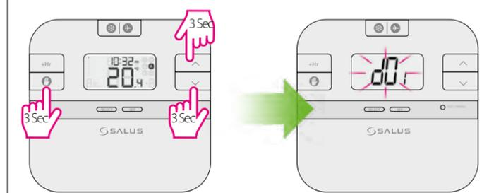
Press the three buttons together for 3 seconds. Use FHR to select dxx parameter, ^ or v to change parameter value and + to confirm.
