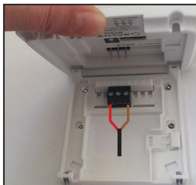
Align the front housing at the top edge.
