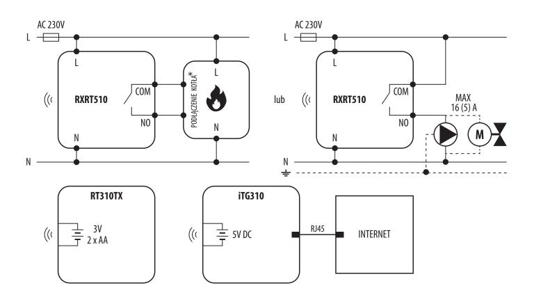
Ξ Battery powered Wireless communication L, N 230V AC power supply Pump Fuse Valve actuator COM, NO, NC Voltage free output Temperature sensor S, S1, S2 Input terminals 3-speed 230V AC fan **LEGEND** SL 230V AC voltage output Light bulb or other load T30NC Contact normally open Thermoelectric actuator (1) Contact normally closed Time programmer NC/COM/NO switch External normally open contact Boiler - Boiler connection \* - Boiler's contacts • 3118 Voltage converter
