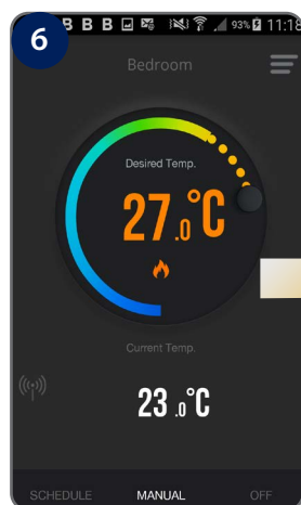
The Flame icon will turn orange and animated meaning the thermostat is calling for heat.
