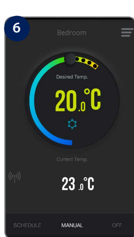
The frost icon will turn blue and animated meaning thermostat is calling for cooling.
