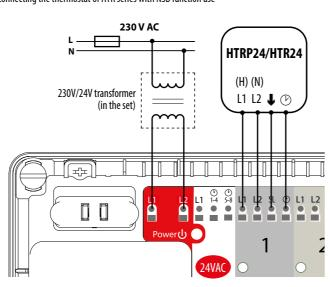
Connecting the RT10 24V thermostat with NSB function use
