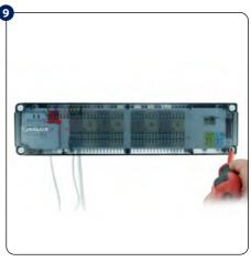
Make sure that all the wires are properly connected, mount top cover and power up the wiring centre - the red power indicator LED will illuminate.
