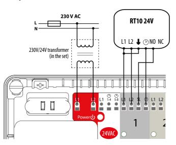
Connecting ON/OFF battery-powered thermostat with voltage-free COM / NO output contacts (e.g. 091FL, RT310, RT510)
