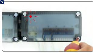
Make sure that all the wires are properly connected, mount top cover and power up the wiring centre - "Power" and "Connection" red LED diodes will light up indicating the correct connection with the KLO8RF 24V wiring centre.
