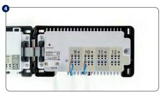
Connect KL08RF 24V and KL04RF 24V using serial connector.
