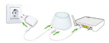
To begin the pairing process the Gateway should be plugged into the power supply and connected to the Internet. Also, make sure that the UGE600 is added to your Salus Smart Home App. For the installation of the Universal Gateway, please refer to the UGE600 manual on salus-manuals.com
