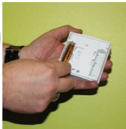
2. Insert the 2 x AA batteries (supplied). If you are installing for the first time please put the thermostat to one side and proceed to page 6.
