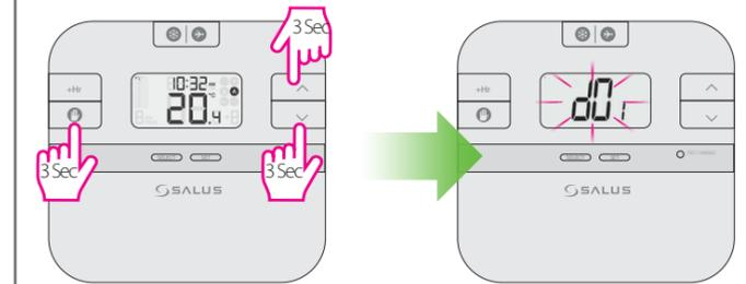
🇬🇧 Press the three buttons together for 3 seconds. Use **SET** to select dxx parameter, ^ or v to change parameter value and **SELECT** to confirm.
