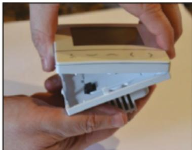
Carefully remove the front housing.
