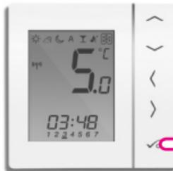
Press tick to confirm the temperature that has been set to.
