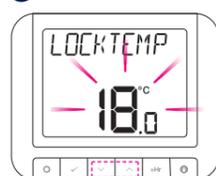
Using UP or DOWN, select the lock temperature and then press SELECT.
