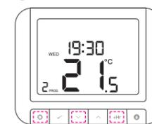
To reset the thermostat, press MENU, DOWN and BOOST simultaneously for 5 seconds.
