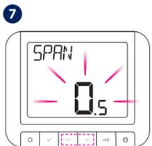
Using UP or DOWN, select the Span value.
