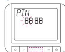
Using UP or DOWN, enter the PIN code number. Press SELECT to confirm every digit.
