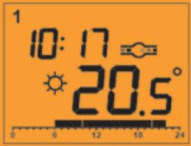
The image shows a digital display with an orange background. At the top left is a small '1'. The main display shows the time '10:17' and a sun icon. Below the time is a valve symbol with an open channel, indicating it is open. The temperature '20.5°' is shown in large digits. At the bottom is a horizontal bar graph with markings at 0, 6, 12, 18, and 24.                 | Wenn der TK geöffnet ist wird dies durch eine "Durchfluss" Animation dargestellt.    |
