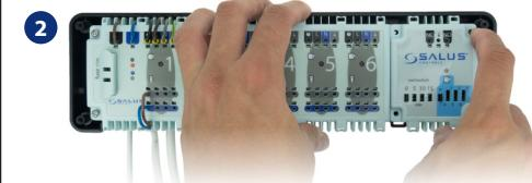
**EN:** Connect the module to the serial connector.
