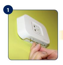
Use a thin object (such as a paper clip) to press and hold the SYNC button on the bottom of the iT500RX receiver for 5 seconds.
