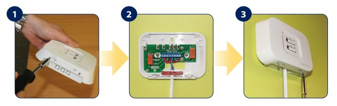
Loosen the screws at the bottom of the receiver unit and unclip the front of the unit.
