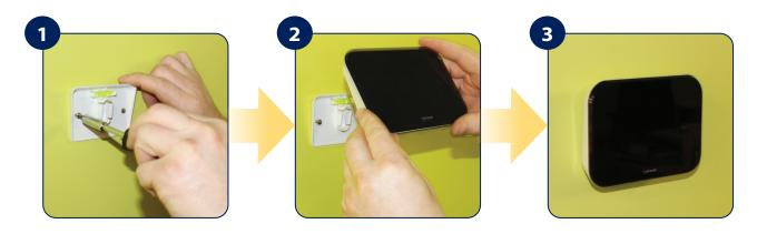
Attach the wall mounting bracket to a suitable wall using the fittings supplied and the built in spirit level.
