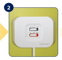
The bottom switch will show a constant red light when iT500RX receiver is ready to pair. Now go to iT500TR thermostat.
