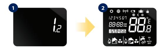
To power on the thermostat you have to put in batteries, then display will show firmware version number...
