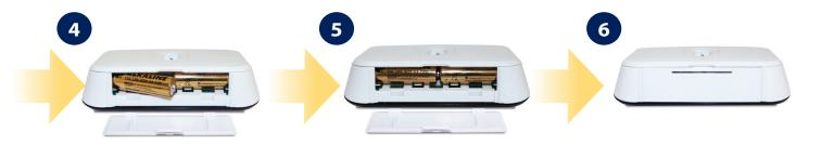
Insert the second battery supplied into the left hand side of the base of the iT500 Thermostat.
