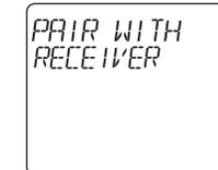
Turn the receiver OFF and ON twice to reset. Ensure receiver switches are ON and AUTO. Red LED should be flashing. Enter thermostat MENU and scroll down until you see the "PAIR WITH RECEIVER" option. Select YES to proceed with Pairing.
