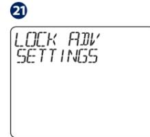
This option will allow you to lock your advanced settings using your access PIN. Using UP or DOWN, create your lock advanced settings, then TICK to confirm.
