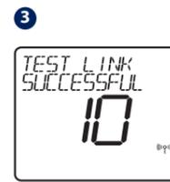
Your thermostat will indicate that the connection has been tested successfully and will return to normal operation.
