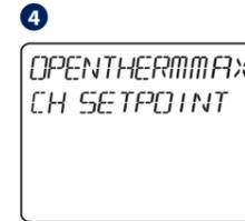
Press TICK to enter menu. Using UP or DOWN, set the maximum opentherm central heating temperature.
