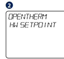
Using UP or DOWN, navigate to HW SETPOINT and press TICK.
