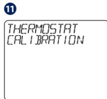
If you think that the temperature displayed on the thermostat is not accurate due to its location, you can calibrate it using this menu with values between -3.5 / +3.5 degree.
