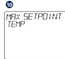
Using TICK, then UP and DOWN you can set the maximum and the minimum room temperature.
