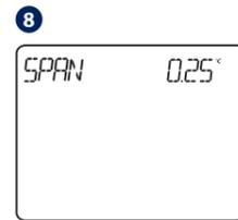
This is a simple ON/OFF algorithm control based on the set point. Using UP or DOWN, you can select the SPAN value. Press TICK to confirm or DOWN to go to next option.
