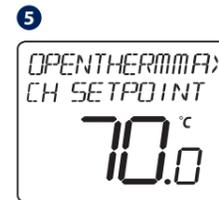
Using UP or DOWN, set the value then press TICK for 3 sec to confirm and exit to main screen.
