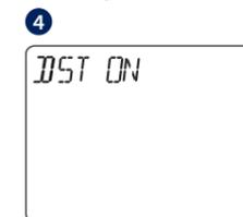
Using UP or DOWN, select ON or OFF. Press TICK to confirm.
