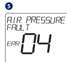
AIR PRESSURE FAULT ERROR
