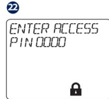
Using UP or DOWN, enter the PIN code number. Press TICK to confirm every digit.
