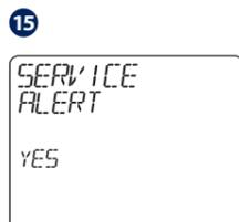
Using UP or DOWN, you can select YES and press TICK to confirm, or you can select NO and go to point 20.
