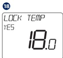
Using UP or DOWN, select the lock temperature and then press TICK.
