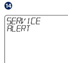
Press TICK to allow installer or landlord to set service reminder and lock temperature level.
