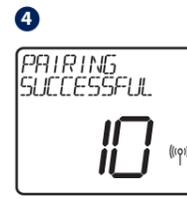
Upon connecting to the receiver, the thermostat will display the message "PAIRING SUCCESSFUL" and return to normal operation afterwards. The red LED will stop flashing when the pairing is successful.
