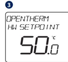
Using UP or DOWN, adjust the temperature and then press TICK.
