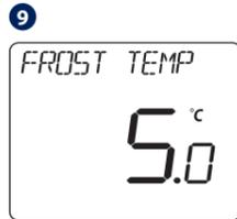
Using TICK, then UP and DOWN you can select FROST value. (5 - 17 degrees C). Press TICK to confirm or DOWN to see the next option.
