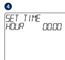
Using UP or DOWN, set the hour and then press TICK, which will then move to minutes, that can be changed in the same way.
