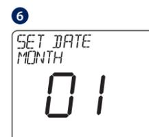
Using UP or DOWN, set the month and then press TICK, which will then move to days, that can be changed in the same way.
