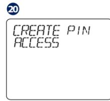
Allows you to create a PIN which may be used to limit access to your settings. Using UP or DOWN, create your PIN access, then TICK to confirm.
