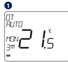
This screen display will be displayed when OT is connected. To change the settings for DHW and/or CH - press MENU and go to ADVANCED SETTINGS.
