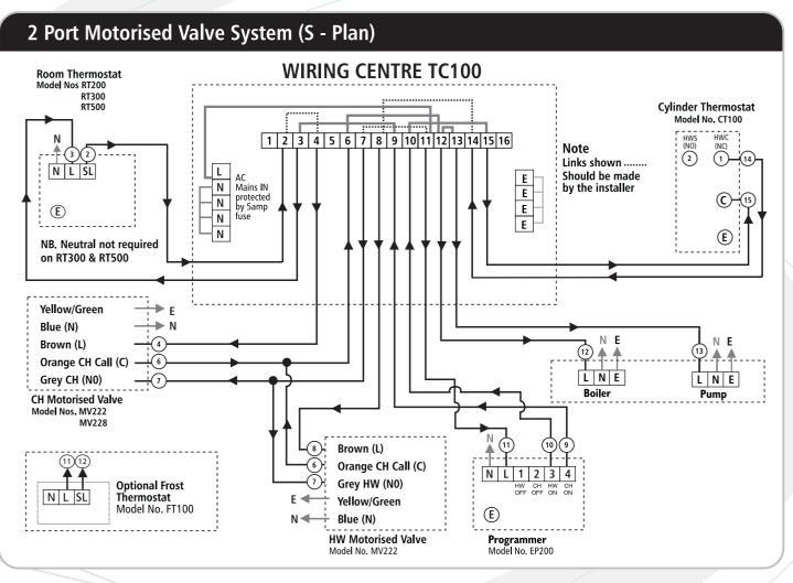
Note: links shown on diagram should be made by the installer.
