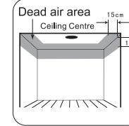
The preferred location to install the smoke detector is in the centre of the ceiling because smoke, heat and combustible products rise to the ceiling and will laterally spread. Keep at least 30 cm distance from lights and decorations and at least 15 cm distance from walls and corners.
