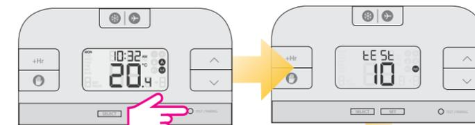
**i** When enter test pairing mode, after a 10 minute countdown the thermostat will time out.
