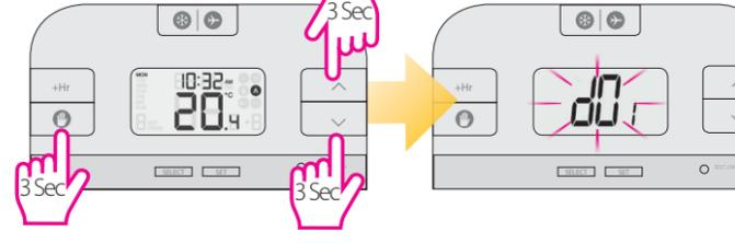
Press the three buttons simultaneously for 3 seconds.
