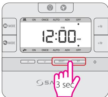
Press and hold the indicated buttons together for 3 sec.
