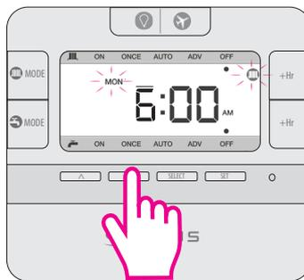
The CH icon and Mon will start flashing. Press up arrow 2 times.
