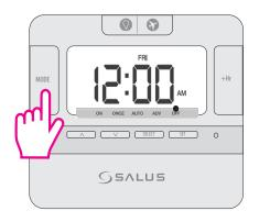
Pressing the Mode key 4 times activates the OFF Mode. In OFF mode, the controller gives the boiler the OFF command, so the heating or the hot water will be turned off.
