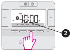
Press Up or Down to set start time for prog 2. Press Select to confirm.
