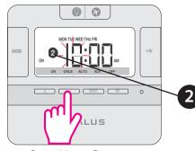
Press Up or Down to set start time for prog 2. Press Select to confirm. Once you have finished setting the start/end time for the first program, the device will jump into the second program, and then into third and afterwards into Sat-Sun. Please follow the same steps for each of the 3 programs. Press **SET** at any time to confirm the setting and return for program set selection.
