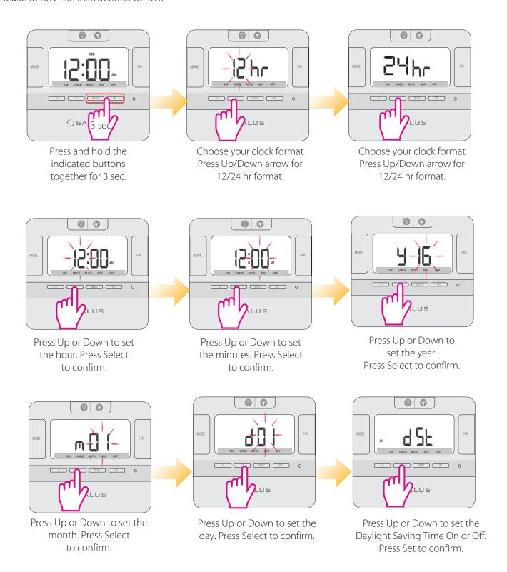
When Daylight saving time is enabled, the clock will automatically change from Greenwich Mean Time (GMT) to British Summer Time (BST) on the last Sunday in March. The clock will automatically change back to GMT on the last Sunday in October.
