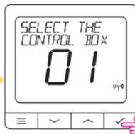
Using and buttons select the Control Box number (press PAIR button on the Control Box to see its address number). Press button to confirm
