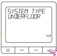
Select system type: UNDERFLOOR, press button to confirm
