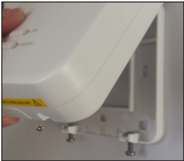
Align the front housing at the top edge.
