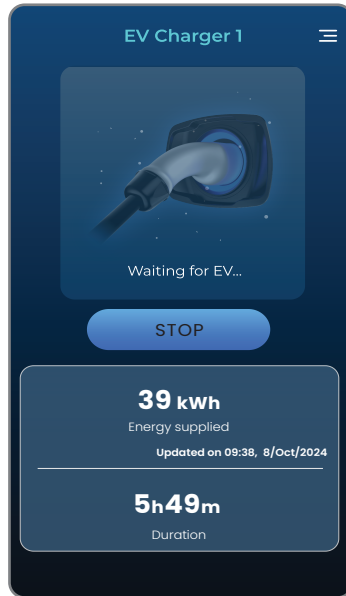
This screen will appear when EV chargers stops or suspends receiving charge.
